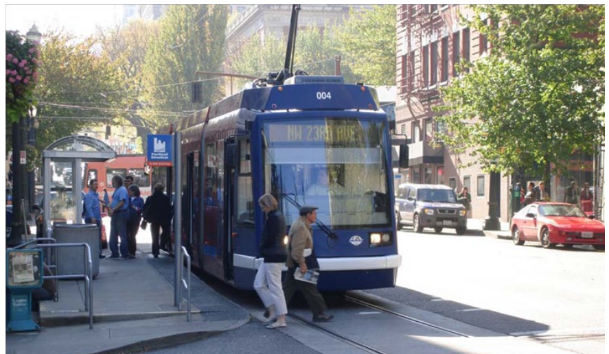
Figure 3.3 Modern Streetcar. Modern Streetcars run in mixed traffic, like buses, and are accessed from streetside stops.
