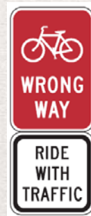
Signs R5-1b and R9-3c Source: Manual on Uniform Traffic Devices (MUTCD)
