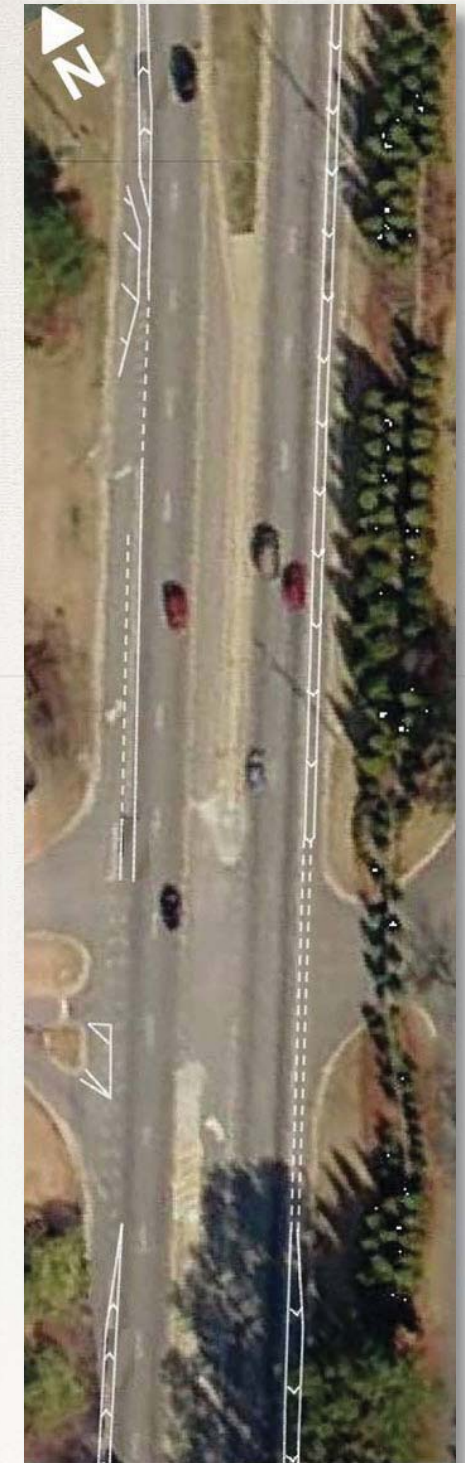
Medlock Bridge Road Road Buffered Bike Lane Concept Source: Sprinkle Consulting, Inc., Fulton County GIS (background aerial)
