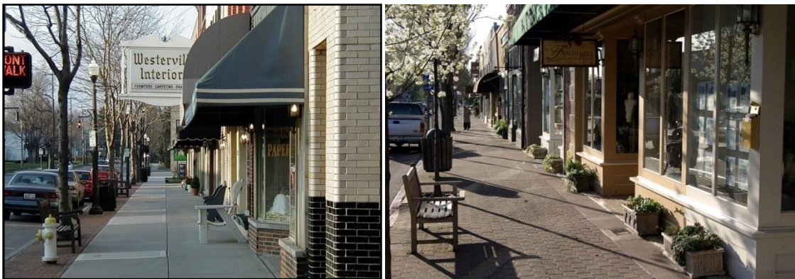
Figure 6-2: Sidewalks with Buffer, Pedestrian and Frontage zones.
