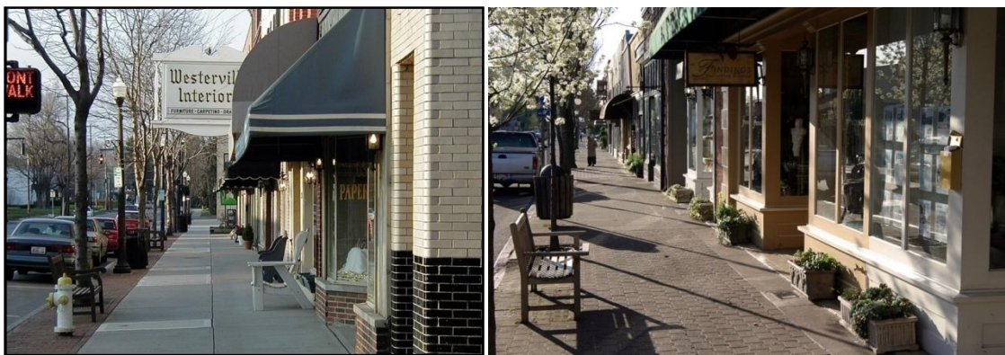
Figure 6-2: Sidewalks with Buffer, Pedestrian and Frontage zones.
