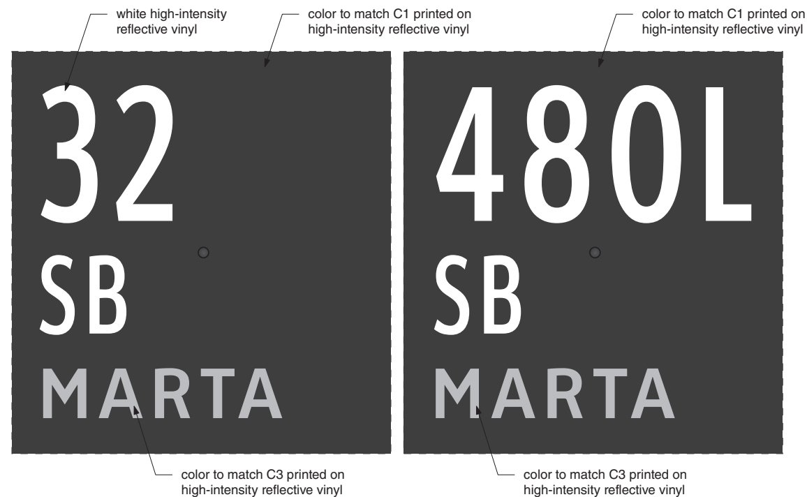
5 Alternate Route Single Panels (Two Panels) Scale: HALF
